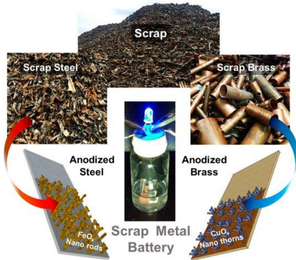
Figure 1. Schematic representation of the process of developing the scrap metal battery with a photograph of one of two scrap metal jar batteries powering a blue LED.
